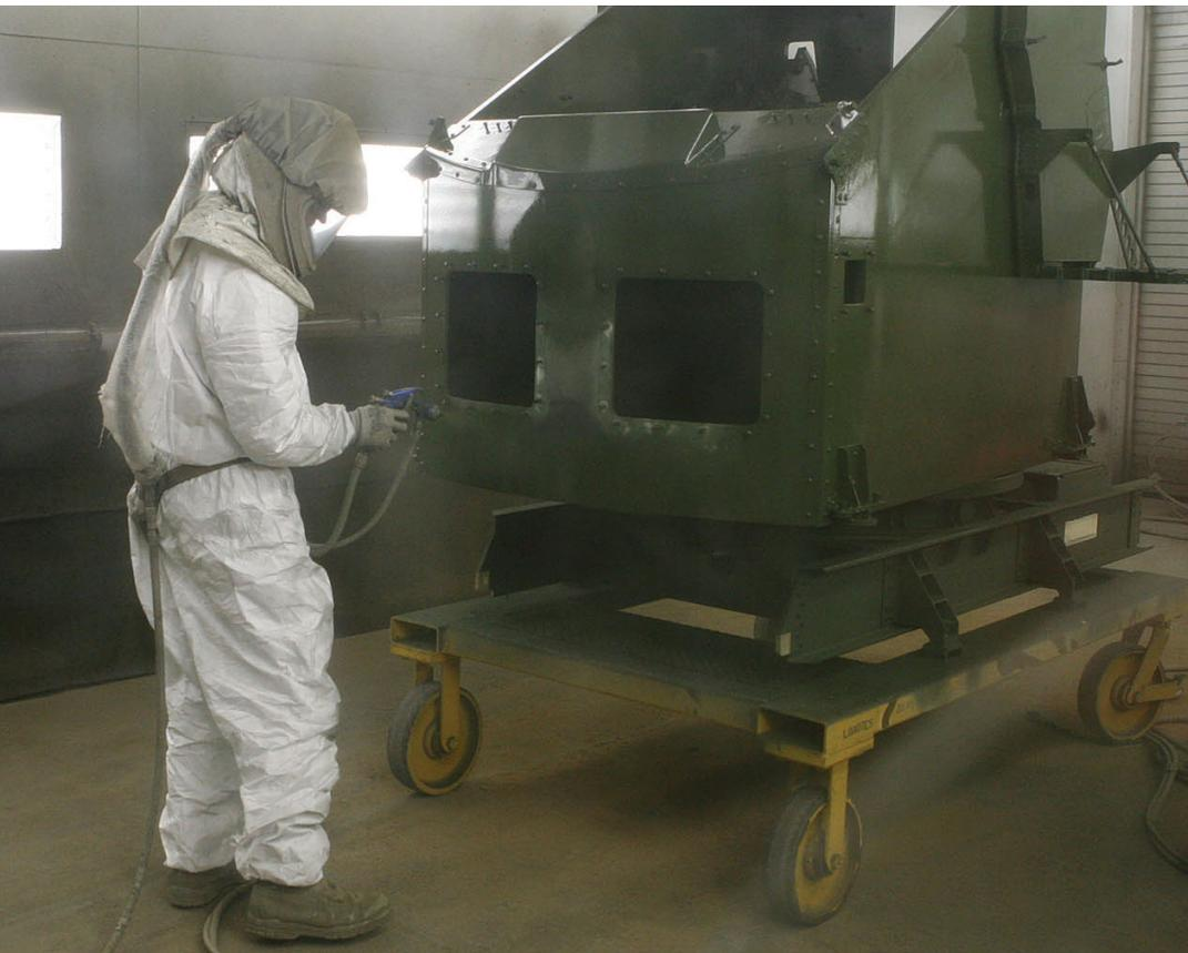
*Using a high volume, low pressure paint gun, a depot painter sprays chemical agent resistant coating over an AN/TWQ-1 Avenger gunner's turret. Letterkenny's advanced paint mixing system reduces labor, cost, and waste. The materials used are at the lowest volatile organic compounds (VOC) that still meet the military specifications and are more environmentally friendly.*
